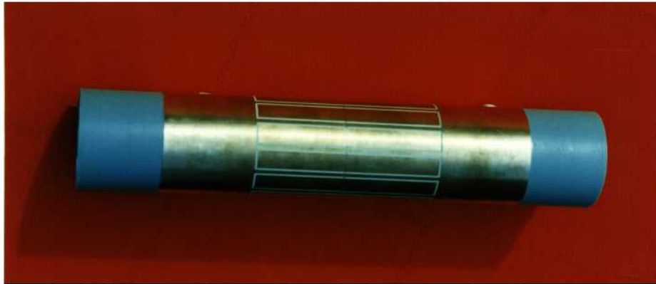
Pipe with sensor electrodes
